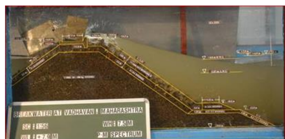
Revised breakwater cross-section and Wave flume studies for the design of revised breakwater cross-section for the proposed development of Port at Vadhavan, Maharashtra
