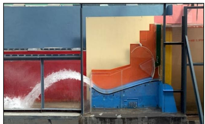
Performance of Spillway with partial gate operation
