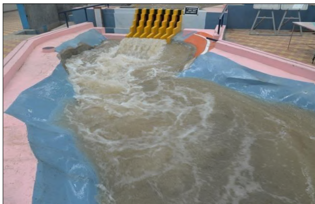
Flow Condition for Gated Operation of Spillway, Q=13000 m 3 /s (100%) at FRL El. 755 m
