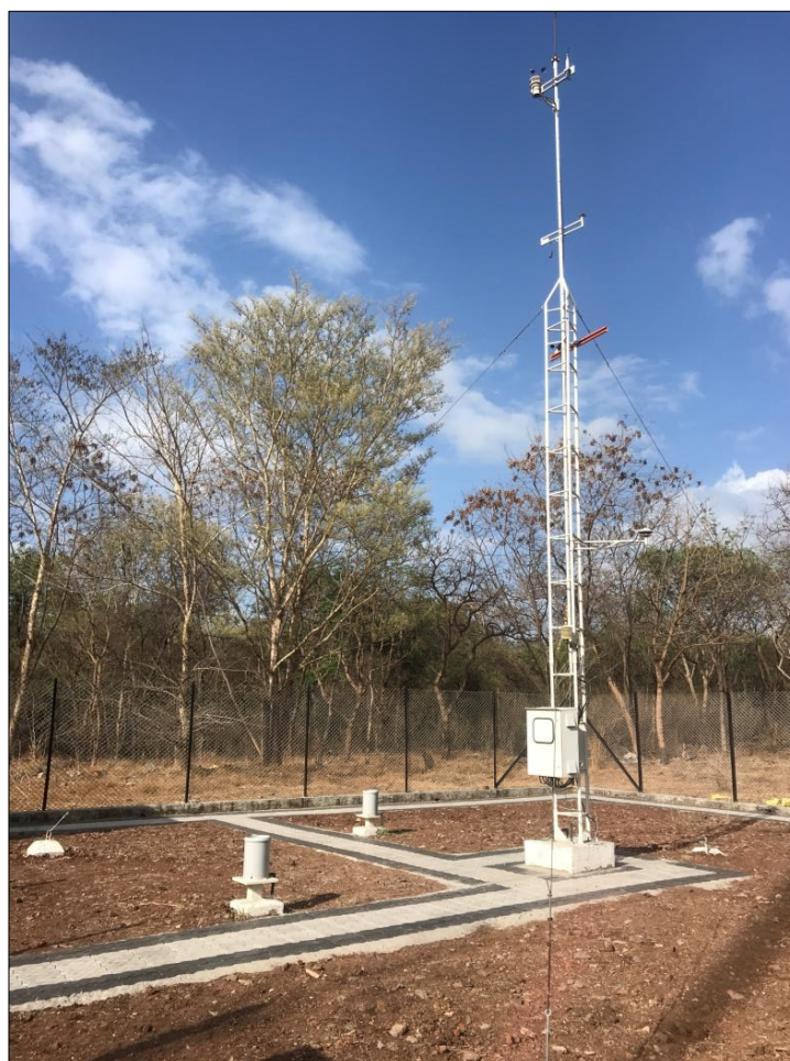
Reference AWS station for Testing & Training purpose as per World Meteorological Organization (WMO) guidelines
