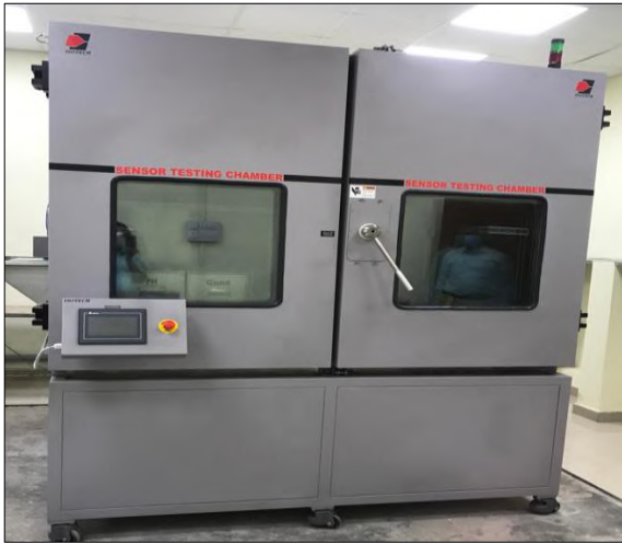
Set up for Environmental Chamber with moving arms for Testing of Water Quality Sensors
