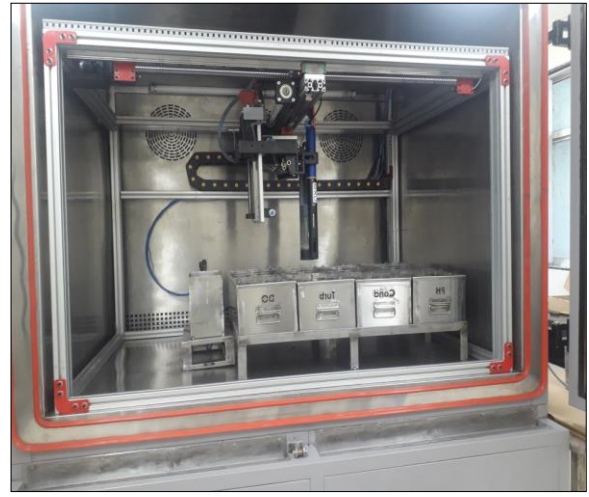
Set up for Environmental Chamber with moving arms for Testing of Water Quality Sensors
