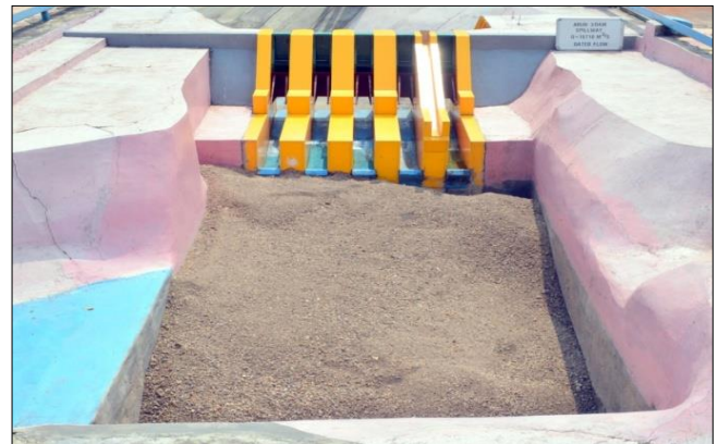
Scour d/s of Spillway for Q = 15,710 \text{ m}^3/\text{s} (Gated operation of Spillway)
