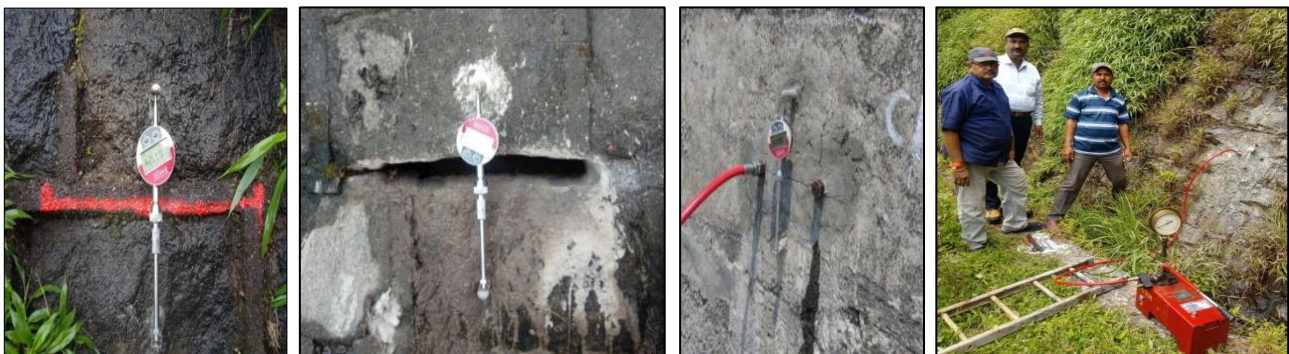
Flat Jack test sequential set up
