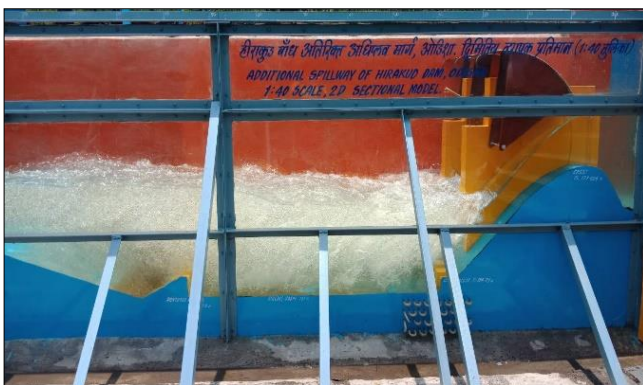
Flow condition downstream of spillway for Ungated Operation of Spillway for the Discharge of 9122 m 3 /s (100%) at RWL El. 191.45 m
