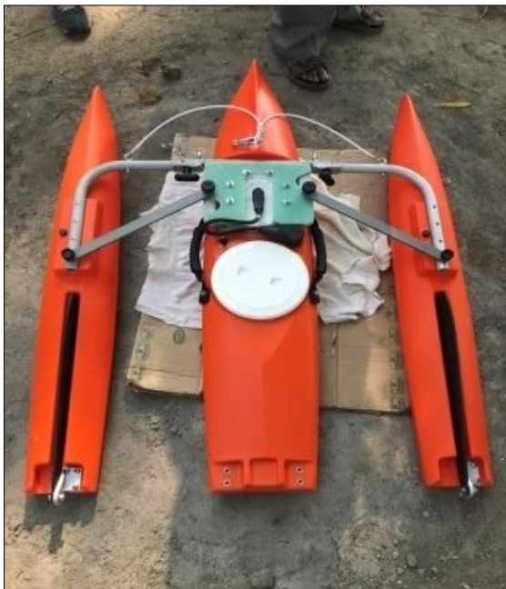
Flow measurement carried out at Ukai HEP by using ADCP
