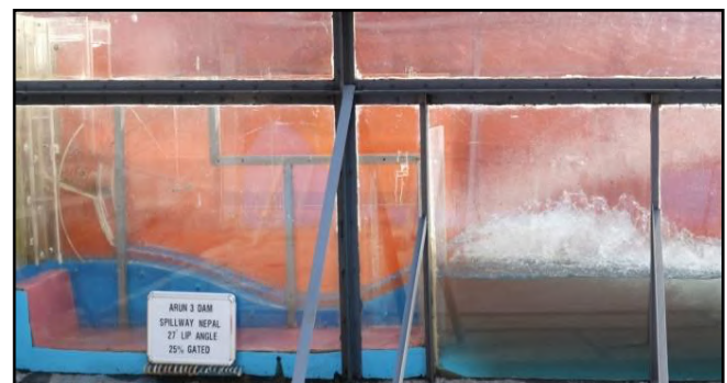
Performance of spillway and energy dissipator for 25% of design discharge with gated operation of spillway
