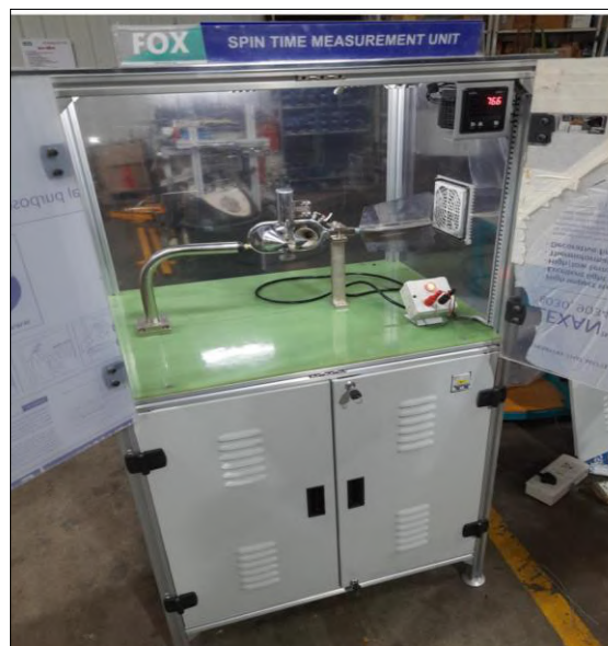
Current meter trolley- Spin time measurement unit
