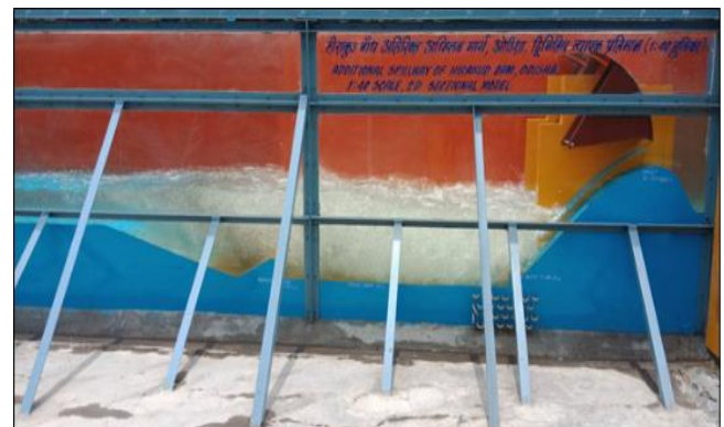
Performance of Stilling Basin for Gated Operation of Spillway for the Discharge of 4561 m 3 /s (50%) at FRL El. 192.024 m
