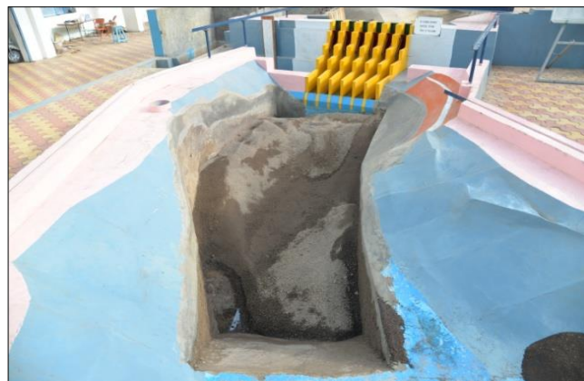
Scour Pattern for Gated Operation of Spillway, Q=13000 m 3 /s (100%) at FRL El. 755 m
