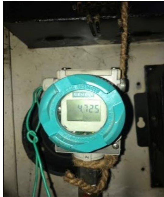
Head measurement carried out at Ukai HEP by using pressure transmitter
